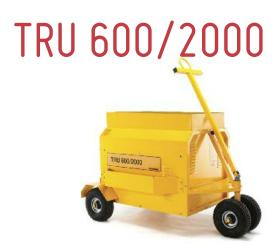
The Powervamp TRU600/2000 is an advanced transformer rectifier unit delivering 28.5V at 600A continuous and 2000A peak for engine starting. Regulation is achieved using additional thyristor control BEFORE the transformer, to achieve a clean output with less ripple than traditional TRUs. The TRU600/2000 is capable of worldwide operation as standard from the factory.
